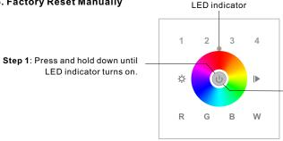
Note: All configuration parameters will be reset after the remote is reset or removed from the network.
