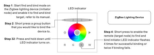
Note: Each remote can bind max. 30 lighting devices.
