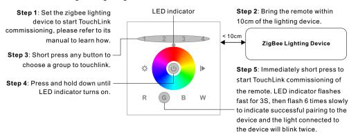
Note: 1) Directly TouchLink (both not added to a ZigBee network), each remote can link with 30 devices.
