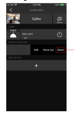
From your ZigBee controller or hub interface, choose to delete or reset the remote as instructed, indicator flashes 3 times quickly to indicate successful removing.
