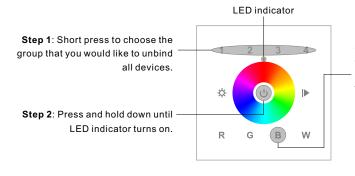
Step 3: Short press 5 times continuously to clear all bound lighting devices. LED indicator flashes 4 times for successful unbinding.
