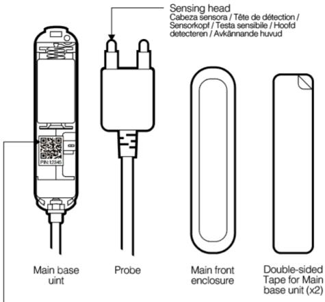
Note: QR Code used for SmartStart inclusion. DSK Code can be found on packaging. Do not remove or damage them.
