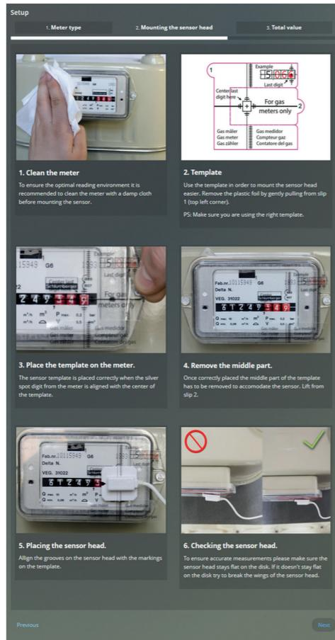
The **sensor head** will partially obscure the numbers - so **write down** the consumption first.
