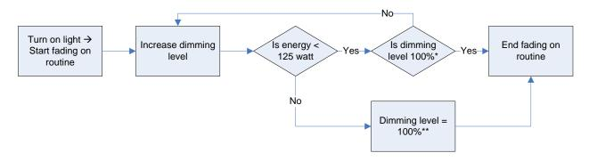
\*In this flowchart the set dimming level is 100%, this can be any other dimming level. However the same routine applies. \*\* When the 125 watt barrier is reached this will be the new 100% dimming level regardless of the set dimming level.
