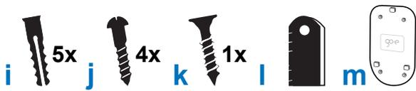
i Dowel 8 x 40 mm   j Screws for wall bracket 4.5 x 50 mm
