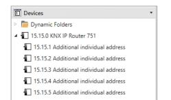
Each individual KNX address can be changed by clicking on the list entry and typing in the desired address into the "Individual Address" text-field. If the text-field frame switches to color red after entering the address, the address is already taken within your ETS project.
