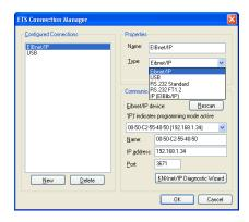
The KNX IP Router 751 supports up to 5 simultaneous connections. For each connection a separate individual address is used. The first additional individual address is assigned by the ETS. By clicking on the 'Settings' at the selected connection "Local Settings" this dialogue box with a corresponding input field appears:
