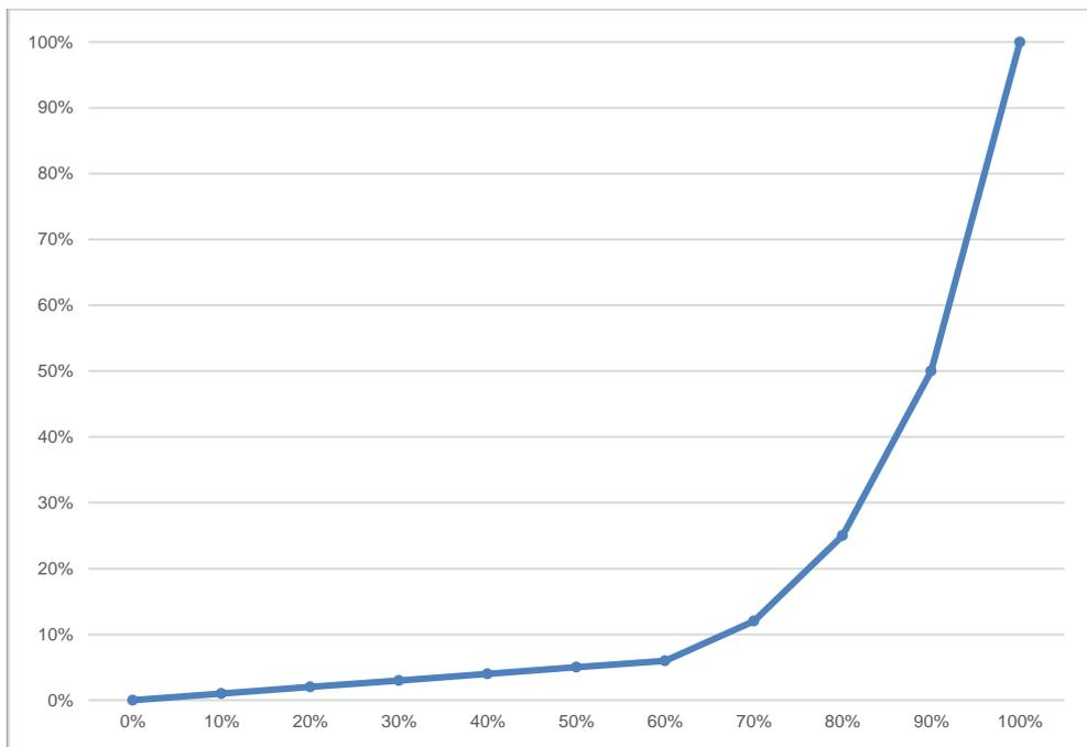
For the dimming curves “Linear” and “Logarithmic” the output values are fixed, for “User defined” they can be freely configured.
