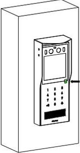
Installation is completed, please remove the protective film.
