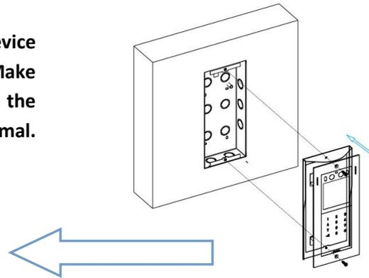
Combine the flush-mounting bracket and flush-mounting rain cover. Then align the fixing holes of flush-mounting bracket with the fixing holes of flush-mounting box, and use torx wrench to tighten flush-mounting plate with two M4x16 torx head screws.
