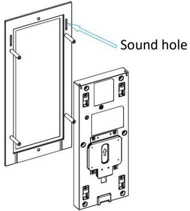
Combine the device with the flush-mounting bracket according to the direction indicated in the figure.
