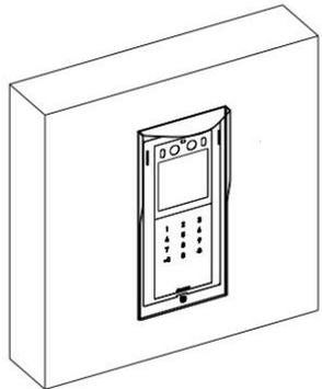
Check if the gap surrounding the device is even and securely installed. Make sure to reserve a gap and power on the device to check the device is normal. Installation is completed.
