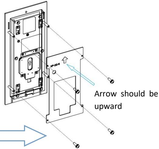
Align the fixing hole of flush-mounting plate with the bolts of flush-mounting bracket, then insert flush-mounting plate onto the flush-mounting bracket. Use four M3x8 crosshead screws to fix flush-mounting plate.
