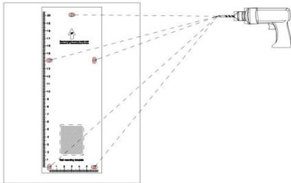
Stick the wall-mounting template onto the wall according to your need. Then use an electric drill with a 6mm diameter bit to make five holes with 20mm depth according to the hole of wall-mounting template.
