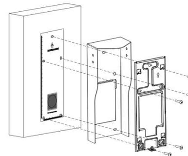
Put the wall-mounting bracket into the rain cover, and please align the bracket's screw holes with the screw holes of rain cover. Then tighten the combined wall-mounting bracket and rain cover on the wall with five ST4x20 crosshead screws.
