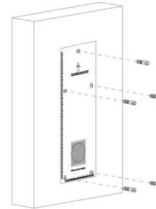
Insert five plastic wall anchors into the holes.
